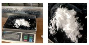
Fig. 2 Polypropylene Fibers used in this study
