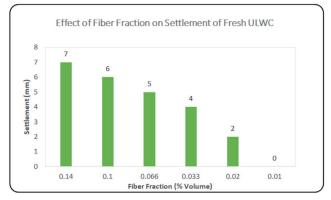
Fig. 16 Effect of fiber volume fraction on the settlement of fresh ULWC specimens
