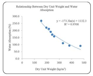
Fig. 10 The relationship between dry unit weight and water absorption characteristics of ULWC specimens produced with P05 aggregate
