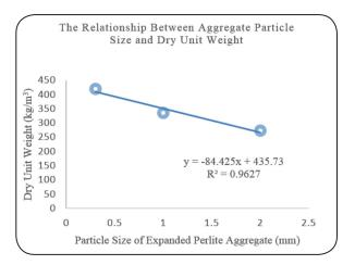
Fig. 13 The effect of different particle size expanded perlite aggregates on the dry unit weight of ULWC specimens.
