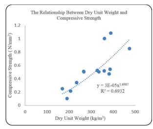
Fig. 11 The relationship between dry unit weight and compressive strength of ULWC specimens produced with P05 aggregate.
