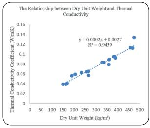
Fig. 12 The relationship between dry unit weight and thermal conductivity coefficient of ULWC specimens produced with P05 aggregate.
