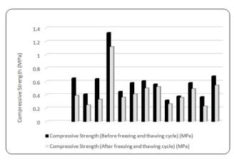
Fig. 18 Effect of freezing and thawing cycles on compressive strength of ULWC specimens
