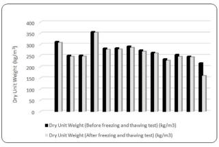
Fig. 17 Mass loss after freezing and thawing cycles
