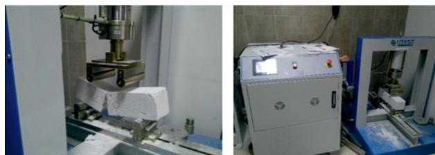
Fig. 6 Tests conducted to determine flexural strength of ultra lightweight concrete specimens
