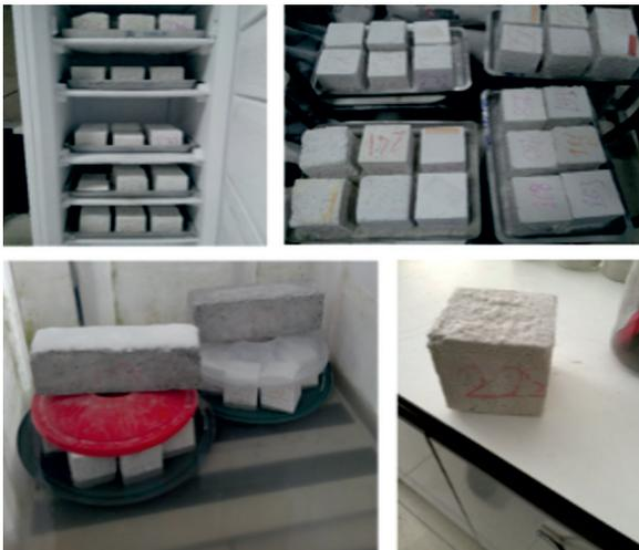
Fig. 8 Freezing and thawing tests of ultra lightweight concrete specimens
