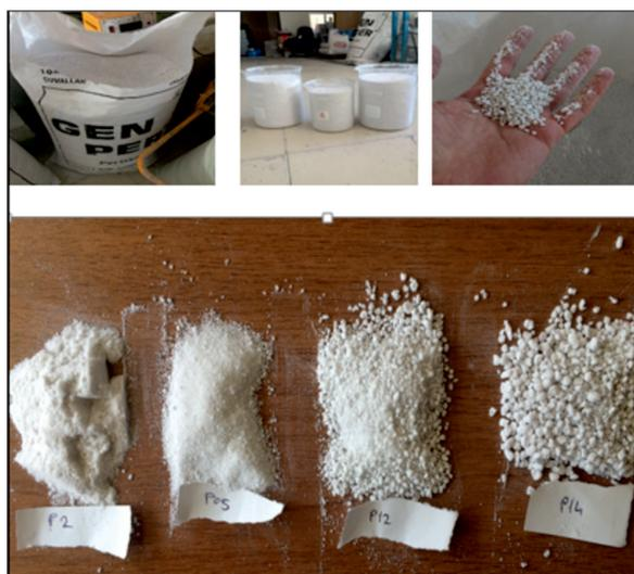
Fig. 1 Different size expanded perlite aggregates used in this study
