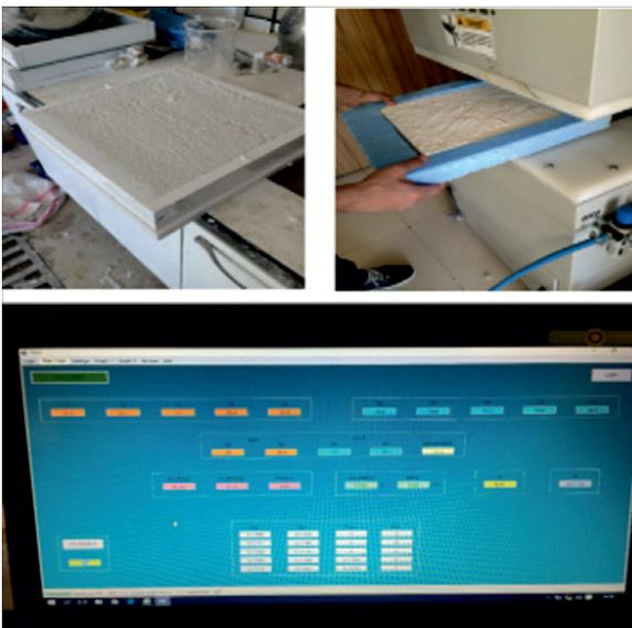
Fig. 9 Thermal conductivity tests of ultra lightweight concrete specimens
