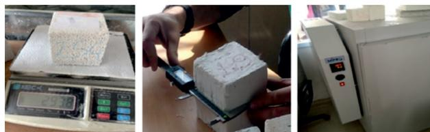
Fig. 4 Determination of dry unit weight of ultra lightweight concrete specimens
