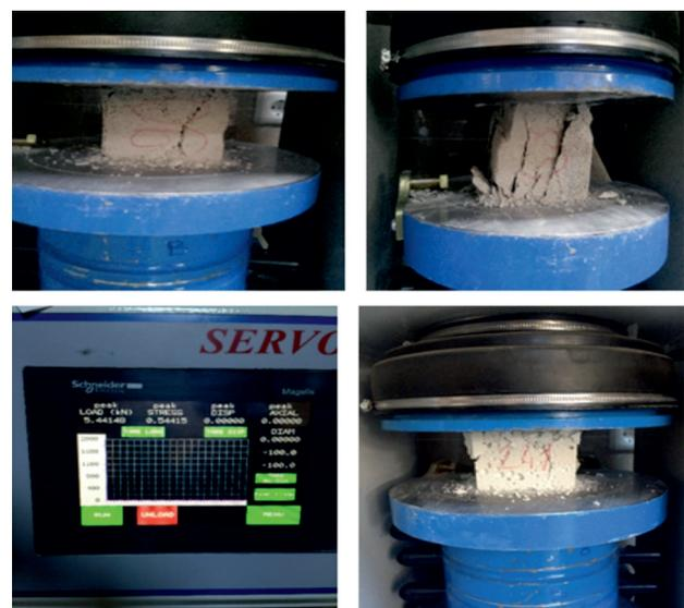
Fig. 7 Tests conducted to determine compressive strength of ultra lightweight concrete specimens
