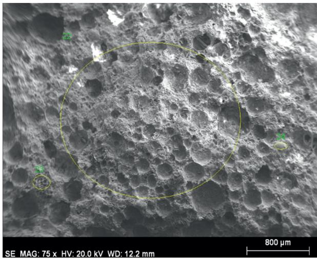
Fig. 15 SEM image of ULWC specimen produced with different size expanded perlite aggregate
