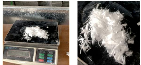
**Fig. 2** Polypropylene Fibers used in this study
