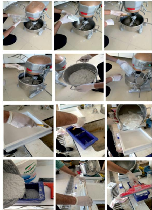
**Fig. 3** Production of ultra lightweight concrete samples using expanded perlite aggregates
