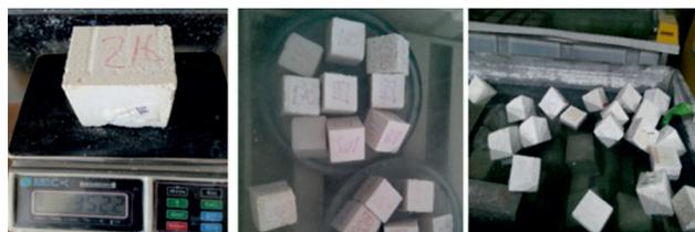
Fig. 5 Tests conducted to determine water absorption of ultra lightweight concrete specimens
