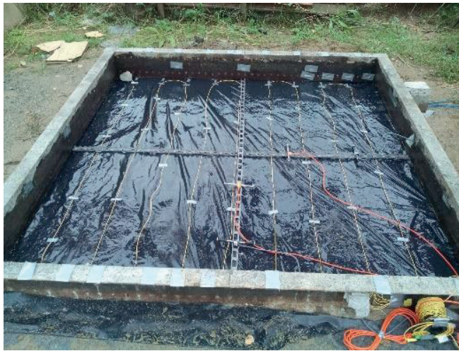
Fig. 17 Location of a strain gages on the fibre concrete slab
