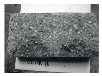
Fig. 14 Water penetration shape of the concrete specimen for Mixture 1
