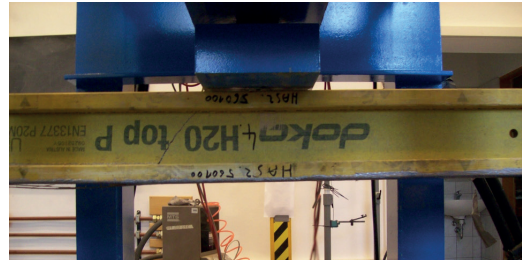
Fig. 10 Failure of a reinforced beam specimen due to shearing in the web
