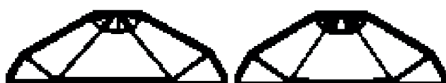
Fig. 4 Design obtained for deterministic, Obj.= 35.6935, (right) and robust design optimization (RDO), Obj.= 25.4565, (left)
