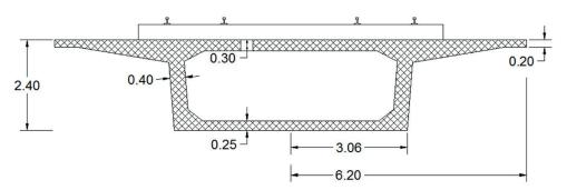
Fig. 2 Cross section of the 24m-span PC box girder (All measurements are in units of m)
