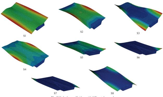
Fig. 9 Mode shapes of bridges with different skew angles
