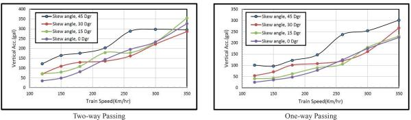
Fig. 16 Deflection and acceleration of the bridge at the entrance quarter-span cross beam section for various skew angles
