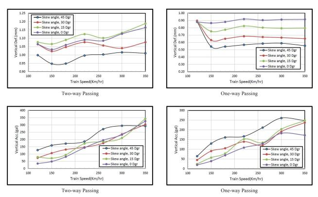
Fig. 18 Deflection and acceleration of the bridge at the outlet quarter-span cross beam section for various skew angles
