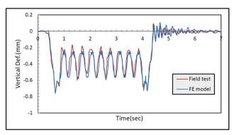
Fig. 7 Displacement time histories of mid-span obtained by numerical model and field tests for the train speed of 260 km/h
