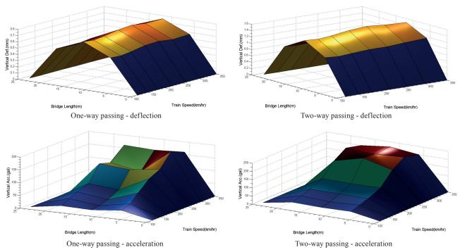
Fig. 11 Maximum acceleration and deflection of the longitudinal center-line for the straight bridge
