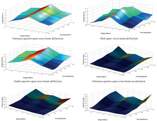
Mid-span- cross beam acceleration
