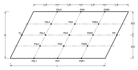
Fig. 8 The target record points in the bridge deck
