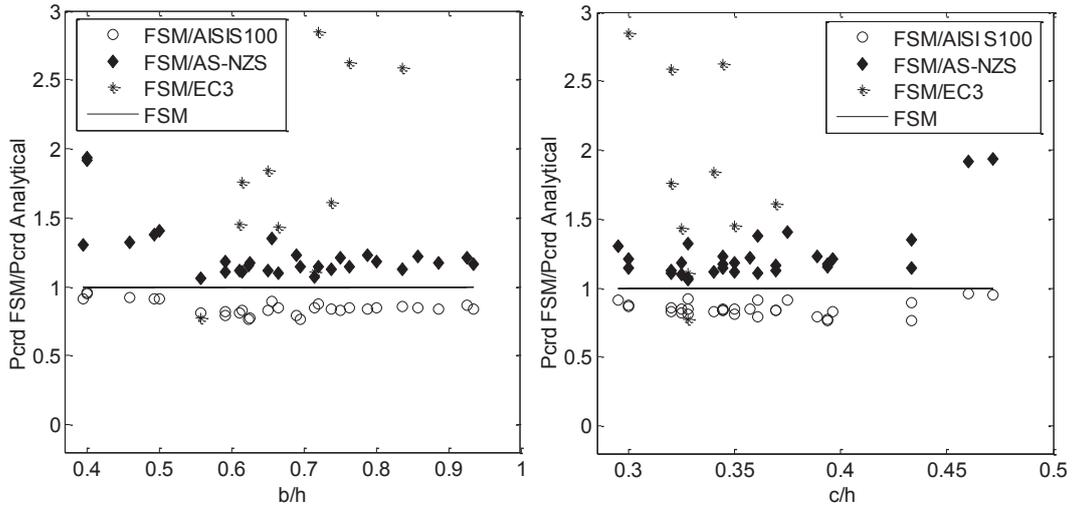
Fig. 13 Comparison of existing analytical models using the numerical results for the fourth zone sections
