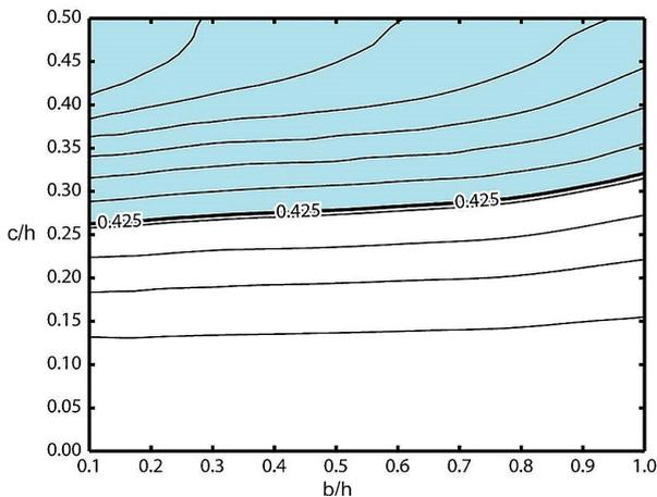
Fig. 5 Probable local buckling zone of the stiffener
