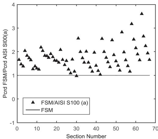
Fig. 19 Comparison of the AISI S100 model results with those given by the finite strip method, for Zone 1
