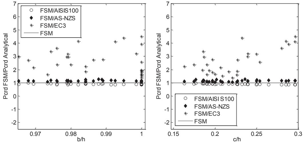
Fig. 16 Comparison of existing analytical models using the numerical results for the seventh zone sections
