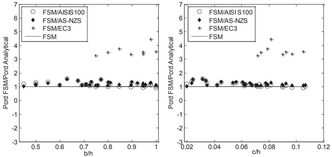
Fig. 14 Comparison of existing analytical models using the numerical results for the fifth zone sections
