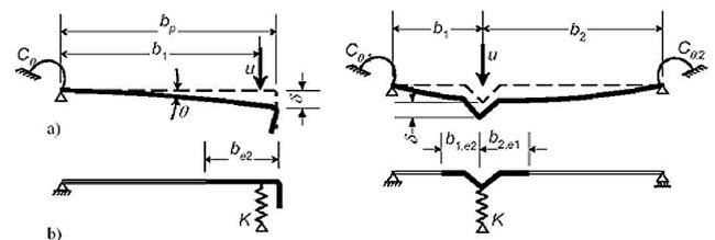
Fig. 3 European standard solution for modeling the distortional instability [25]
