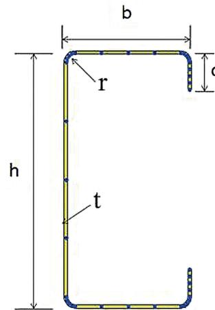
Fig. 9 FSM approach for the rounded-corner model
