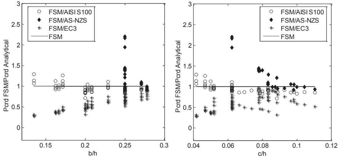
Fig. 10 Comparison of existing analytical models using the numerical results for the first zone sections
