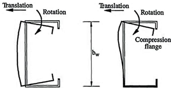
Fig. 1 Distortional buckling mode for a steel member subjected to compression and bending [24]
