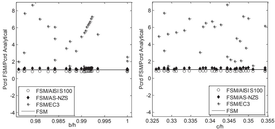
Fig. 17 Comparison of existing analytical models using the numerical results for the eighth zone sections
