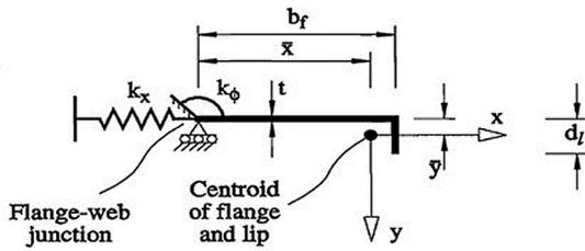
Fig. 2 Analytical model for distortional buckling of lipped flange [21]
