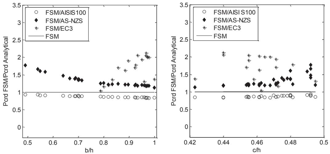
Fig. 15 Comparison of existing analytical models using the numerical results for the sixth zone sections
