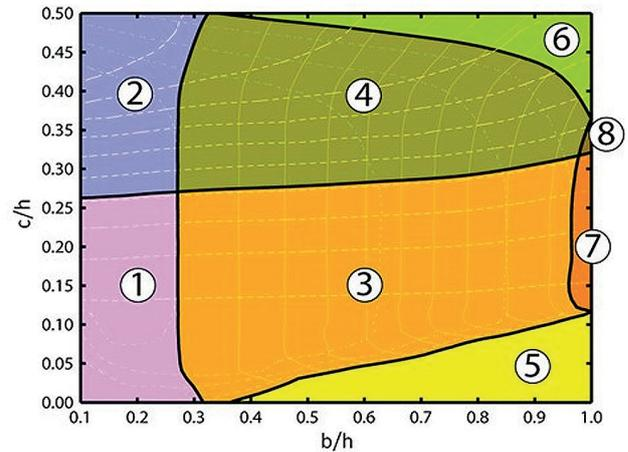
Fig. 7 Zones corresponding to different types of instability of C-profiles subjected to compression
