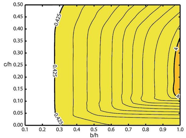
Fig. 6 Probable local buckling zone of the flange
