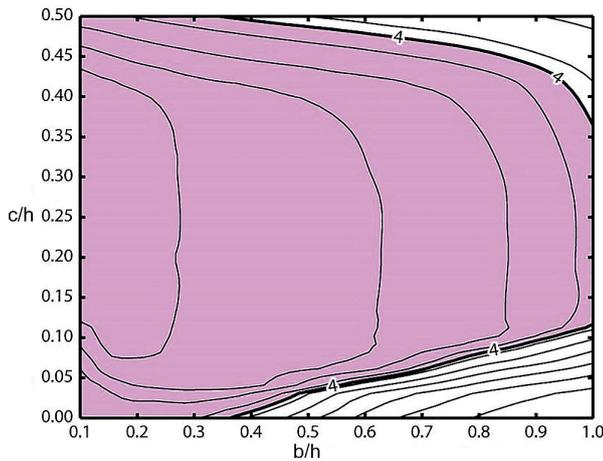
Fig. 4 Probable local buckling zone of the web
