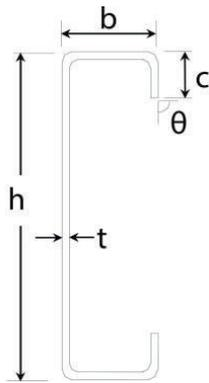
Fig. 8 Dimensions of the C-shaped section
