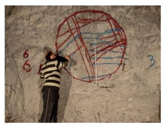
Fig. 1 Surveying Fractures of Rudbar Lorestan dam site using circular scan window
