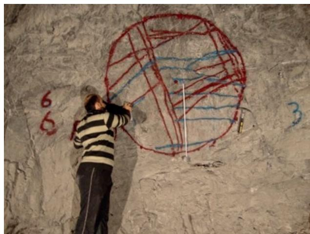
Fig. 1 Surveying Fractures of Rudbar Lorestan dam site using circular scan window
