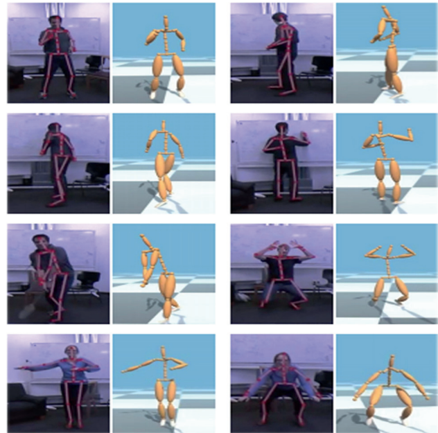
Fig. 1 The real-time 3D pose estimation method provides a natural motion interface, e.g. for sport games (source: [13])
