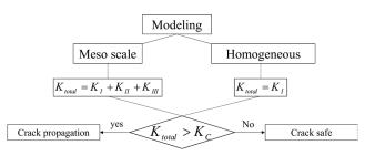
Fig. 18 Effect of modeling type on crack growth
