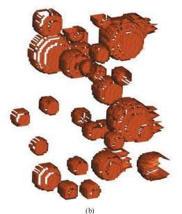
Fig. 9 a) Cement matrix and cement/cement interface; b) Aggregate/ cement interface (ITZ)
