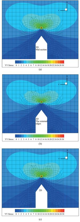
Fig. 4 A comparison of the stress contour along y in the a) 3D and b) 2D modelling: outer aspect, middle plane along the thickness, c) 2D modelling
