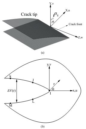
**Fig. 3** a) Stress intensity factor calculation using displacement correlation; b) the opening of the crack plane in the 2Dimensional space
