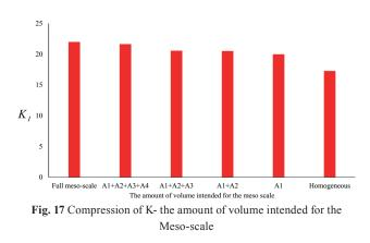
As indicated in Fig. 17, whatever the Meso-scale volume is greater, stress intensity factor is more precise. More important point in the Meso-scale volume selection is computational cost. By an increase in Meso-scale volume, computational cost and degrees of freedom increases dramatically. Given the following results, the same volume limited to 25 mm from each direction of crack plane was selected for the Meso-scale modelling.
