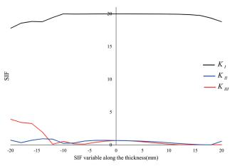
Fig. 12 Stress intensity factor along the numerical sample thickness
