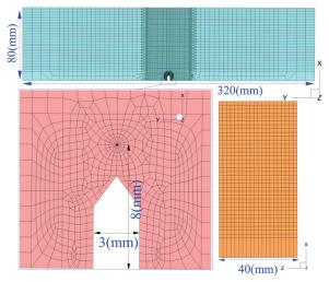
Fig. 2 Model dimensions and the finite element mesh
