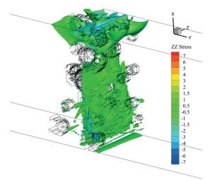
Fig. 11 ZZ stress, the concentration of the stress generated around aggregate along the thickness
