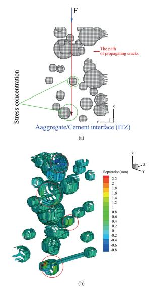
Fig. 14 a) Prediction of crack prediction; b) separation ITZ zone
