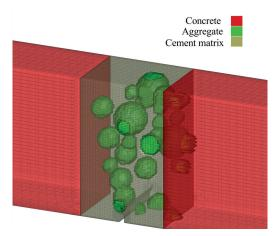
Fig. 7 One example of aggregate distribution and Meso-scale limited volume
