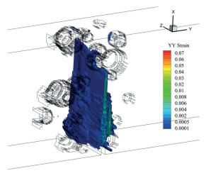
(b) Fig. 10 YY strain a) Forward view; b) Back view
