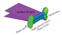
Fig. 5 Tri-axial stress conditions along the thickness
