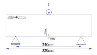
Fig. 1 Geometry of experimental concrete beams subjected to threepoint bending [13]
