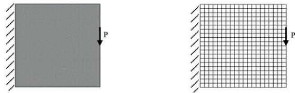
Fig. 5 Design domain: cantilever beam plus exemplary FE mesh
