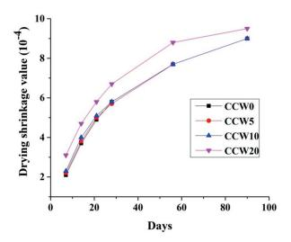
Fig. 4 Drying shrinkage of mortar with various whisker content
