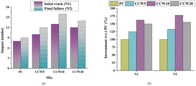
Fig. 8 Impact properties: (a) Impact number; (b) Percentage increase in strength w.r.t PC
