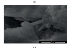
**Fig. 11** SEM images of crack resistance and toughening mechanisms of whiskers: (a) crack deflection; (b) whisker pull-out; (c) crack bridging
