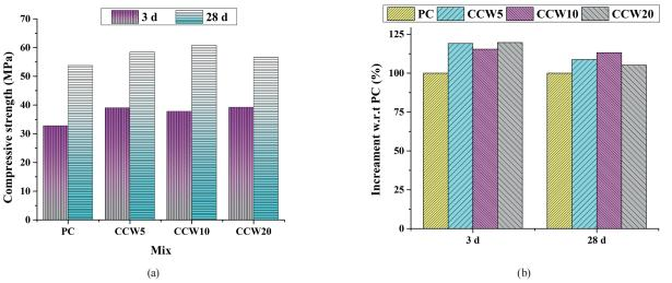
Fig. 5 Compressive properties: (a) Strength; (b) Percentage increase in strength w.r.t PC
