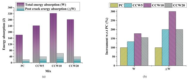
Fig. 9 Impact properties: (a) Impact energy; (b) Percentage increase in strength w.r.t PC
