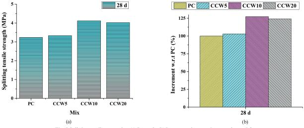
Fig. 7 Splitting tensile properties: (a) Strength; (b) Percentage increase in strength w.r.t PC
