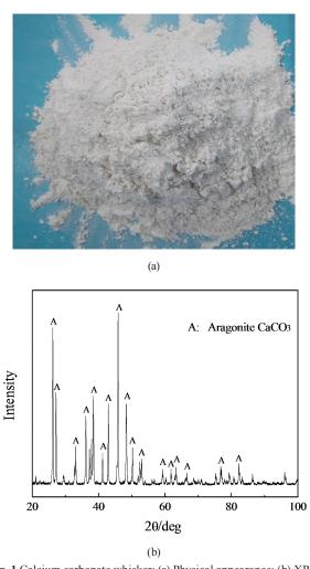
Fig. 1 Calcium carbonate whisker: (a) Physical appearance; (b) XRD pattern
