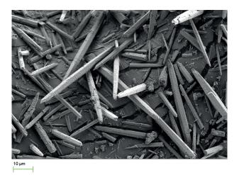
Fig. 2 SEM of calcium carbonate whisker
