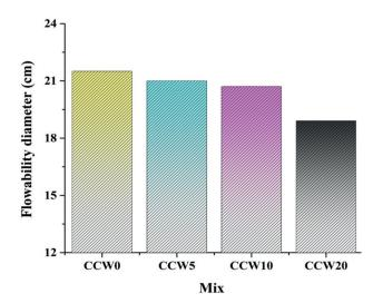
Fig. 3 Fluidity of mortar with various whisker content
