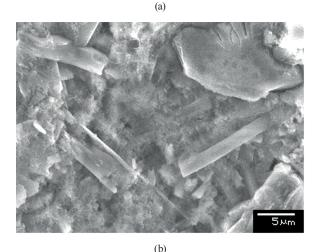
Fig. 10 SEM images of whisker-reinforced cement mortar: (a) whisker bonding; (b) whisker uniform distribution
