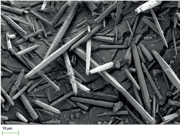
**Fig. 2** SEM of calcium carbonate whisker
