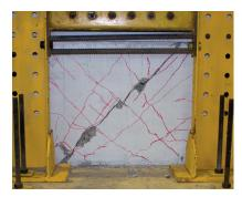
(e) 1.5 % drift Fig. 5 Propagation of damage with drift increments specimen SW1
