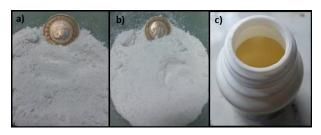
**Fig. 3** Physical appearance of nanomaterials used in this research work, a) Nano-Bentonite, b) Nano-CaCO<sub>3</sub> c) ZycoTherm® liquid antistripping nanotechnology
