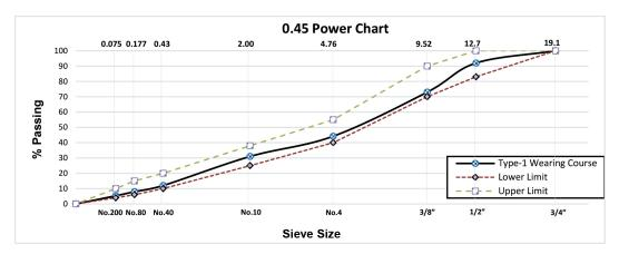
Fig. 2 Limestone 0.45 power gradation chart for the type-1 wearing course
