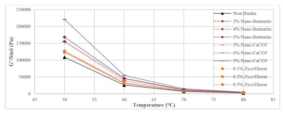
**Fig. 7**  $G^*/\sin\delta$  values for RTFOT-aged samples at 10 Hz
