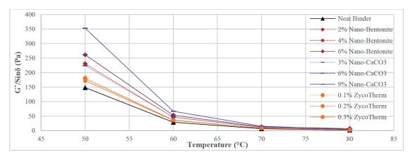
**Fig. 6**  $G^*/\sin\delta$  values for unaged samples at 10 Hz
