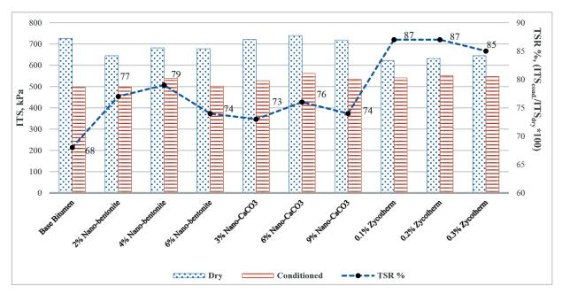
Fig. 8 ITS and TSR results for mixtures prepared with neat and nanomodified binders
