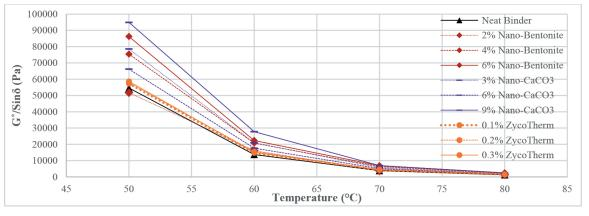
**Fig. 5**  $G^*/\sin\delta$  values for RTFOT-aged samples at 0.01 Hz
