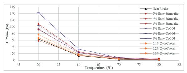
**Fig. 4**  $G^*/\sin\delta$  values for unaged samples at 0.01 Hz
