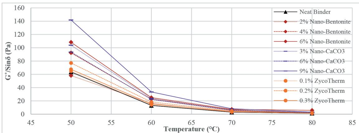
Fig. 4  $G^*/\sin\delta$  values for unaged samples at 0.01 Hz
