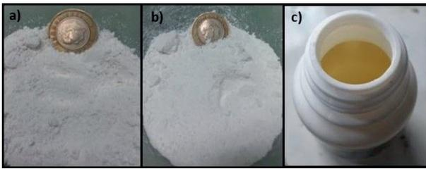
**Fig. 3** Physical appearance of nanomaterials used in this research work, a) Nano-Bentonite, b) Nano-CaCO<sub>3</sub>, c) ZycloTherm® liquid antistripping nanotechnology
