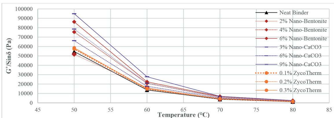
Fig. 5  $G^*/\sin\delta$  values for RTFOT-aged samples at 0.01 Hz
