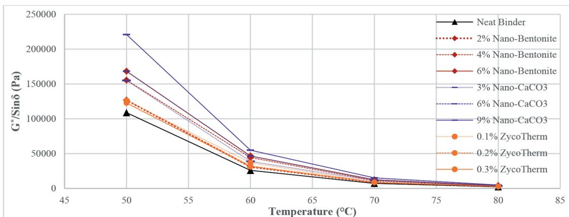
Fig. 7  $G^*/\sin\delta$  values for RTFOT-aged samples at 10 Hz
