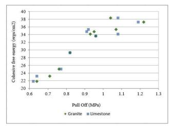
Fig. 12 Pull Off and cohesion free energy
