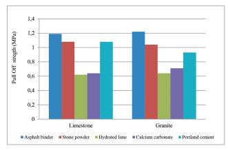
Fig. 5 Tensile strength values on the control asphalt binder and different mastics (AC 60-70)
