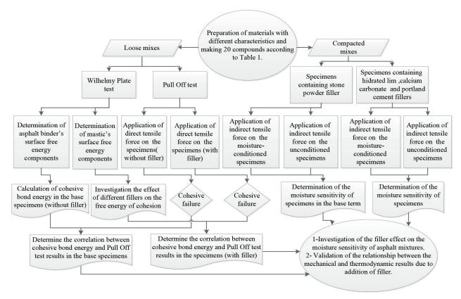
Fig. 2 .Laboratory program flowchart
