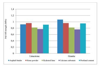
Fig. 6 Tensile strength values on the control asphalt binder and different mastics (AC 85-100)
