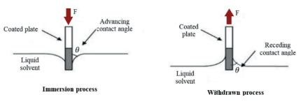
Fig. 4 WP dynamic method for advancing and receding contact angles
