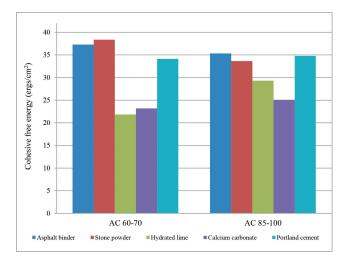
Fig. 11 Values of asphalt binder and different mastics cohesion free energy
