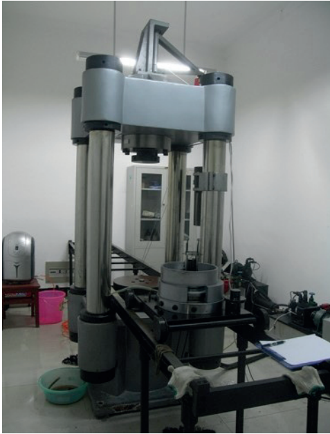
Fig. 3 RLW-2000 creep test machine
