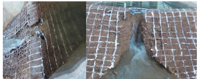
Fig. 3 Breaching process during laboratory test
