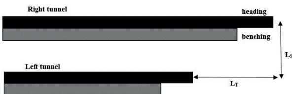
Fig. 8 Schematic spacing between twin tunnels
