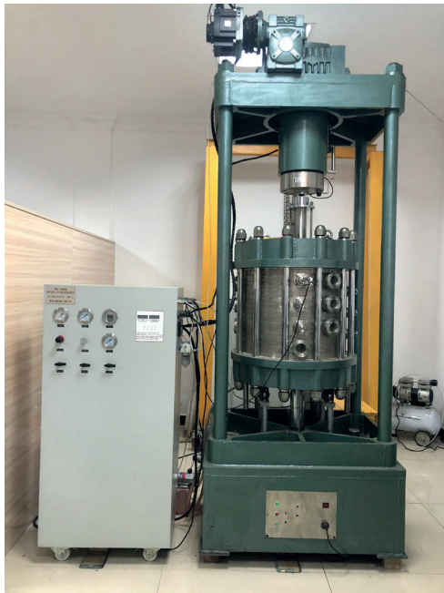
Fig. 3 YRQ-1000 rock soaking-air drying cycle load rheometer
