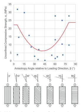
Fig. 2 Inherent anisotropy from unconfined compressive strength (UCS) testing in moderately to highly weathered shales from the Pilbara region of Western Australia
