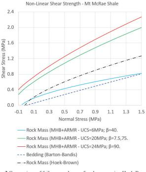
Fig. 3 Comparison of failure envelopes of rock mass using Hoek-Brown and Modified Hoek-Brown criteria with ARMR, and bedding shear strength from Barton-Bandis
