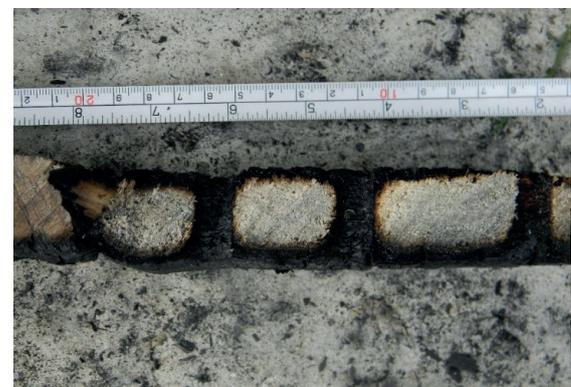
Fig. 11 Discolouration at the screws (made by the Authors)
