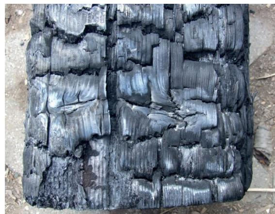
**Fig. 9** Cracks on the carbonized surface (made by the authors)
