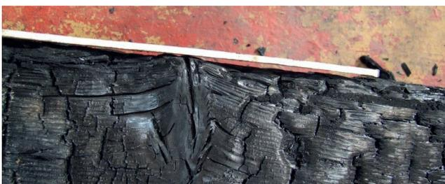
**Fig. 7** A so-called "ditch" recess near the knot (made by authors)
