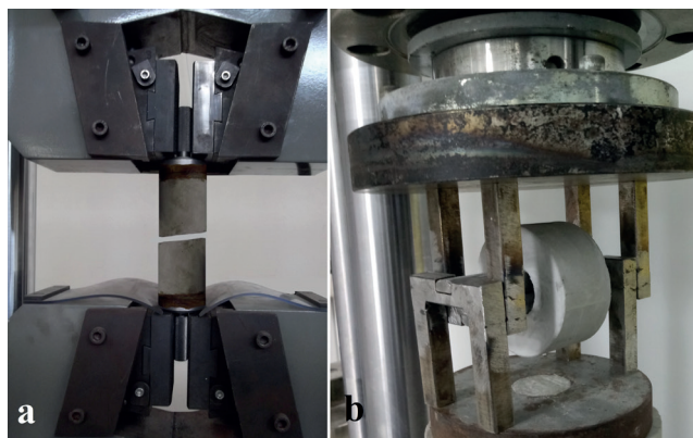
Fig. 4 a) Standard direct tensile strength test, b) DDT test
