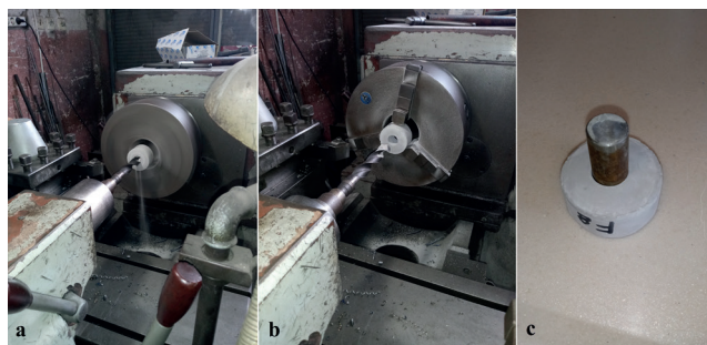
Fig. 3 a) drilling hole, b) a drilled disc, c) a casted disc with hole
