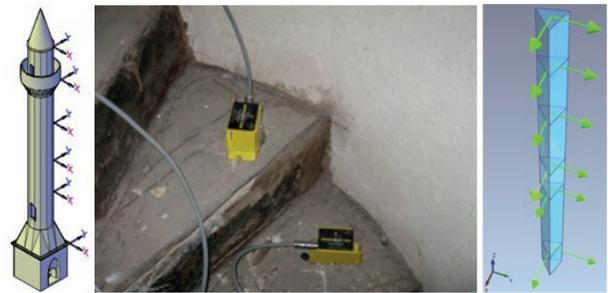
Fig. 6 Locations and directions of the accelerometers on the minaret
