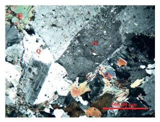
Fig. 10 Intergranular crack with the coalescence wing crack (crossed nikol) – BeR-4\_KV-001
