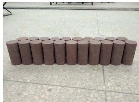
Fig. 1 Standard rock sample after screening and processing
