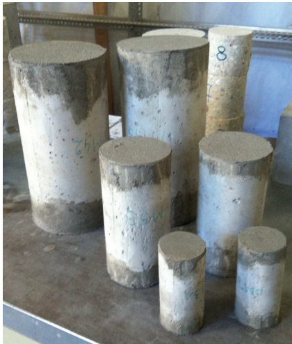
Fig. 3 Cylinder samples ready for compressive testing
