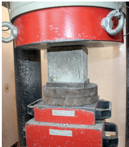
Fig. 4 150 mm cube sample in the Alpha 3-3000 S testing machine
