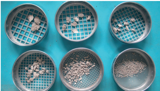
Fig. 6 Rock chips produced by pre-cutting machine cutter
