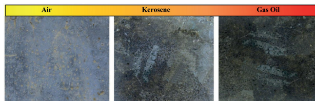
Fig. 3 discoloration analysis of tested RPC specimens before and after exposure to crude oil products
