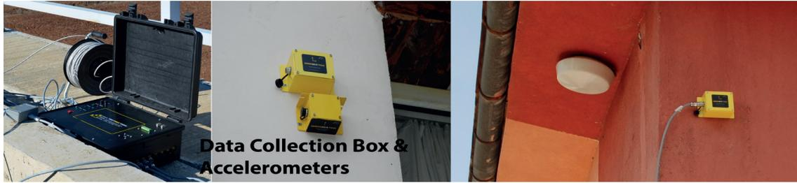
Fig. 2 Data collection box and accelerometers
