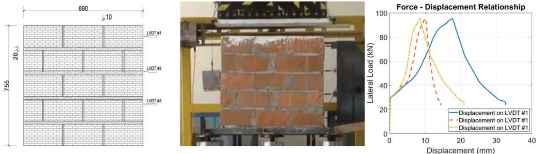
Fig. 8 LVDT placements, loading equipment and the load–displacement values
