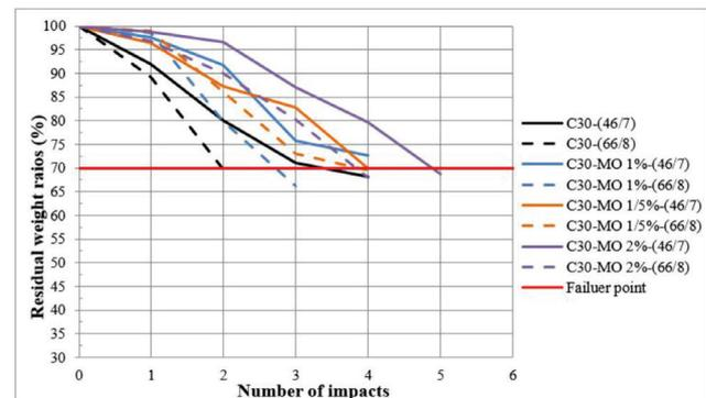
Fig. 11 Residual-to-initial weight ratios of the unwrapped C30 specimens
