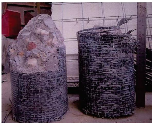
Fig. 6 Rupturing of the CFRP wrapping
