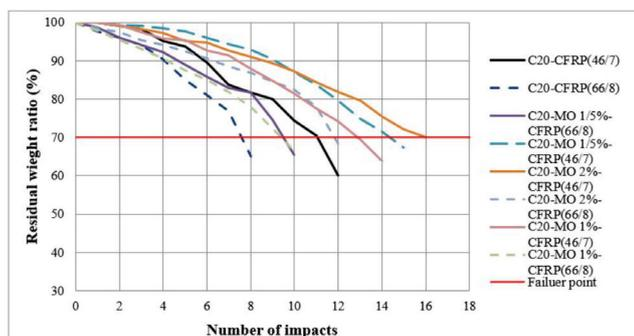
Fig. 10 Residual-to-initial weight ratios of the CFRP-wrapped C20 specimens
