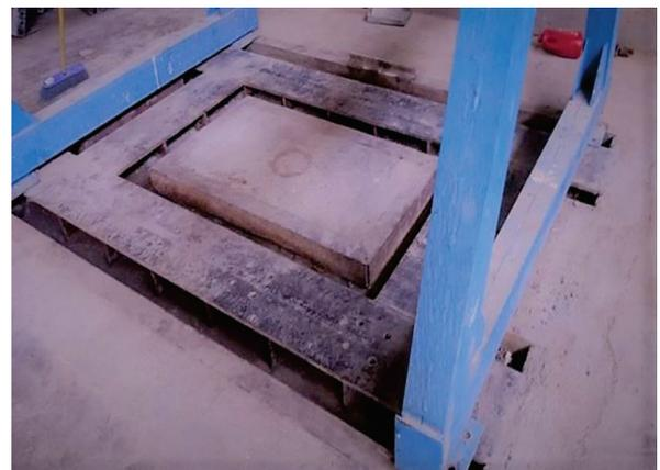
**Fig. 3** Strong floor constructed for the experiments
