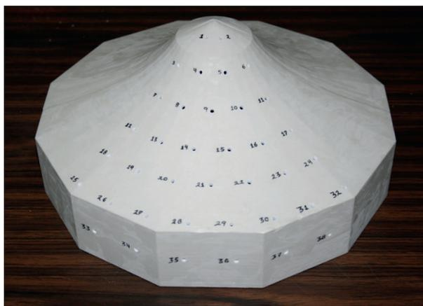
Fig. 6 Scale model and its measurements holes
