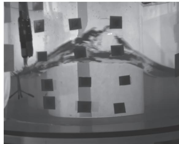
Fig. 5 Single Kelvin wave,  $\bar{h} = 0.0933$  m,  $\tau = 0.0167$ ,  $\Omega = 6.84$  rad/s
