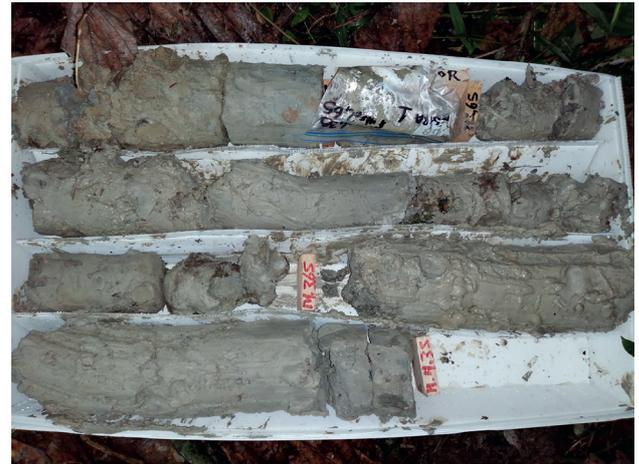
**Fig. 9** The SPT test was performed on this material. This box shows the continuation of the third layer. This layer is where the SPT test was carried out
