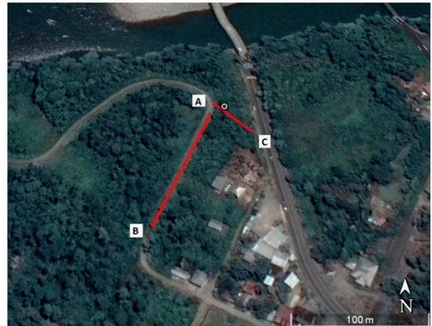
**Fig. 5** The red lines gives the positions of the two seismic lines: SL1 and SL2, used in this study. The dot-mark is the position of the borehole
