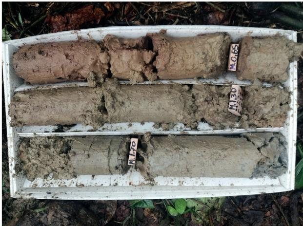
**Fig. 8** Borehole box shows three layers of soil. The first brown layer corresponds to a sandy clay soil (0.0 m to 0.75 m). The second dark brown layer corresponds to a plastic clay, with a low percentage of sand (0.75 m to 1.30 m). The third gray layer corresponds to a clayey sandy material (1.30 m to 4.35 m)
