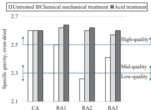
Fig. 4 Oven-dried specific gravity of aggregates used before and after treatments
