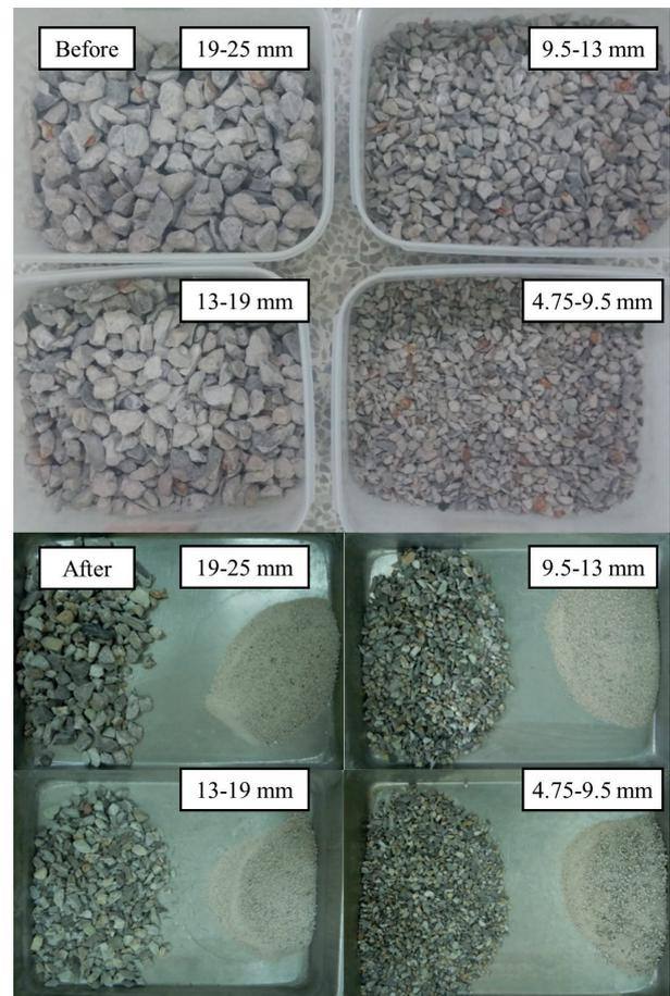
Fig. 2 Recycled aggregate before and after acid treatment
