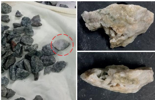
Fig. 6 Natural aggregate damaged by hydrochloric acid
