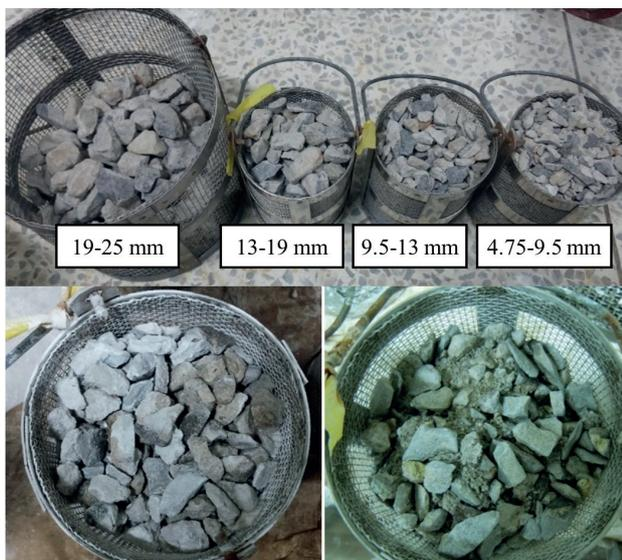
Fig. 1 Recycled aggregate before and after chemical-mechanical stress treatment
