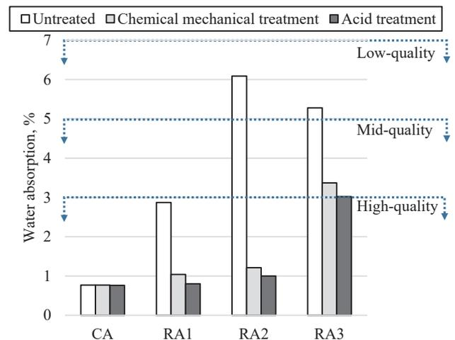
Fig. 5 Water absorption of aggregates used before and after treatments
