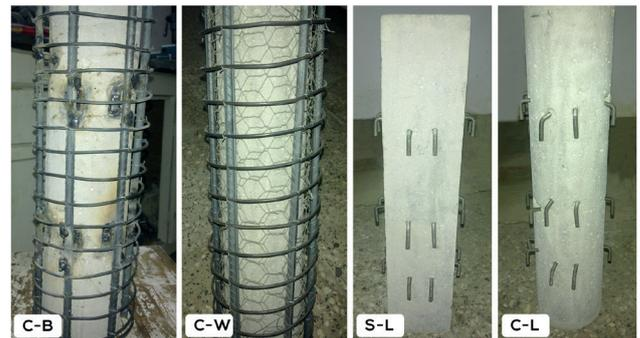
Fig. 6 Connecting elements and different specimens before concreting the casing
