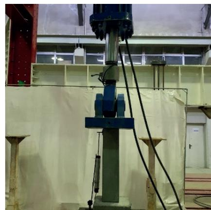
Fig. 7 Test setup for compressive experiments on short RC columns
