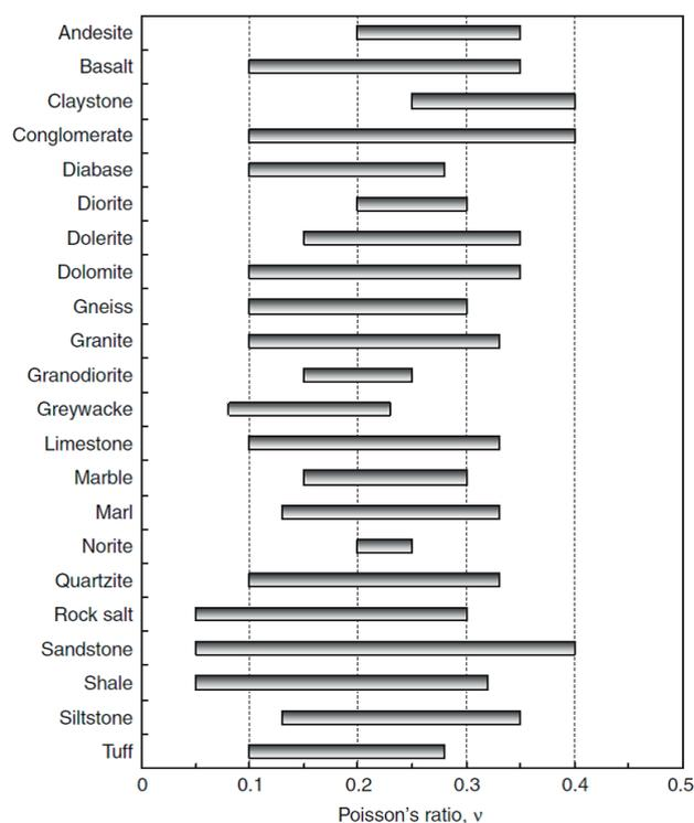
Fig. 1 Typical ranges of values for Poisson's ratio of some rock types (collected by Gercek [1])
