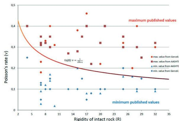
Fig. 2 Poisson's ratio in function of the rigidity of intact rock according to the results of Lógó and Vásárhelyi [4]
