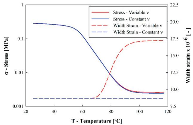
Fig. 4 Comparison of results considering a constant and variable Poisson's ratio. Comparison of results considering a constant and variable Poisson's ratio [6]
