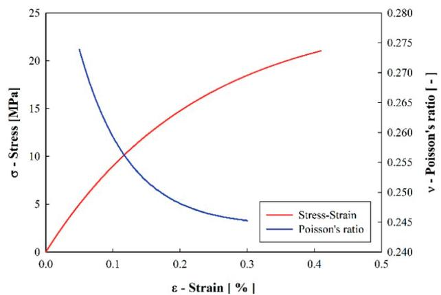
Fig. 5 Experimental tensile strength test [6]
