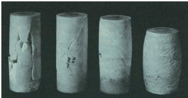
Fig. 7 Marble samples: from unconfined (left) to increasing confining pressure (to right) (according to Kármán [13–14])
