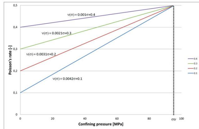
Fig. 10 Changing the Poisson's ratio in case of  $\sigma_c = 100$  MPa and  $m_i = 10$  (using Eq. (25))
