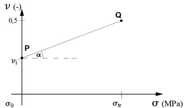
Fig. 9 Poisson's ratio ( $\nu$ ) in the function of confining pressure ( $\sigma$ )
