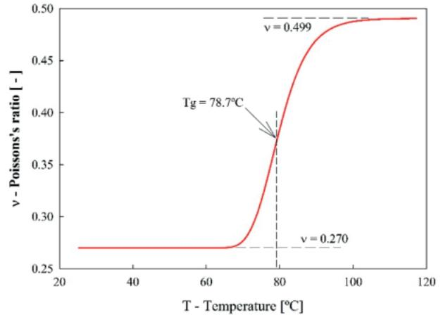
Fig. 3 Connection between Poisson's ratio and the specimens temperature [6]
