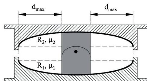
**Fig. 2** Double curved surface slider (DCSS)
