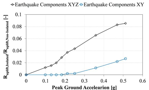
**Fig. 8** Comparison between non-isolated and isolated structure – Column base uplift forces
