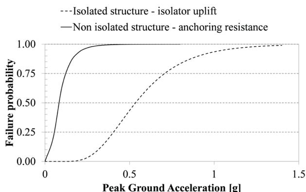
Fig. 10 Comparison of the fragility curves between non-isolated and isolated structure
