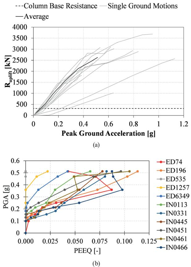
Fig. 6 Incremental dynamic analysis results; (a) IDA curves, (b) Maximum plastic deformations on the non-isolated structure
