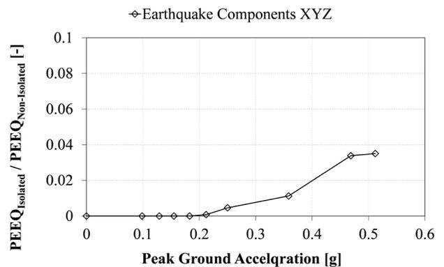
**Fig. 9** Comparison between non-isolated and isolated structure – Average maximum plastic deformations
