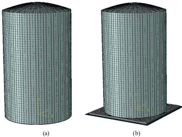
Fig. 4 FE model developed for the investigated gas tank structure; a) Non-isolated Structure, b) Isolated structure
