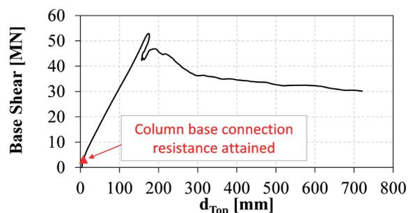
Fig. 5 Push-over base shear-relative roof displacement curve
