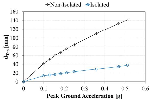
**Fig. 7** Comparison between the non-isolated and isolated structure global deformation (Average relative roof displacement)
