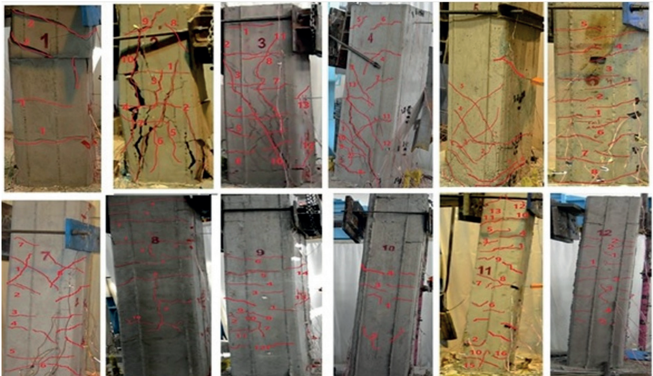
Fig. 10 Cracking patterns of the specimens after failure
