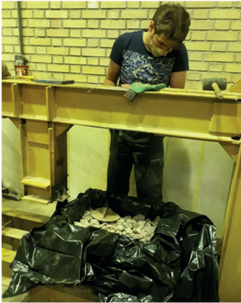
Fig. 10 Compacting ballast layers in shear box in superstructure laboratory
