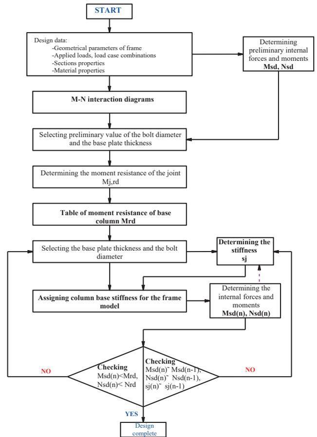
Fig. 3 Flow chart for design semi-rigid base plate connection
