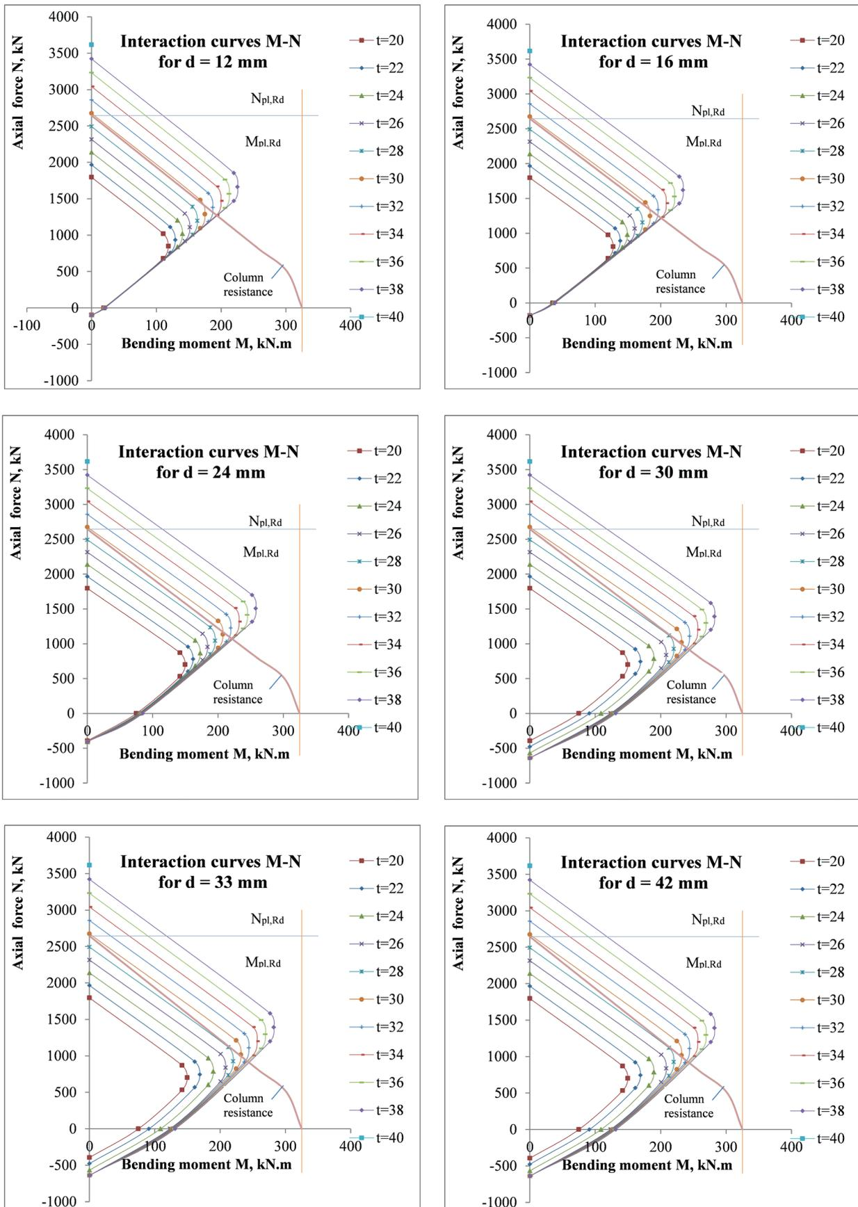
Fig. 7 M-N Interaction diagram for different base plate thickness (Column HEA300,  $f_y = 235$  Mpa; Bolt 4.8,  $n = 4$ ,  $f_{ub} = 400$  MPa; Concrete: C25/30; Base plate,  $e_a = 60$  mm,  $e_b = 80$  mm,  $e_c = 65$  mm)
