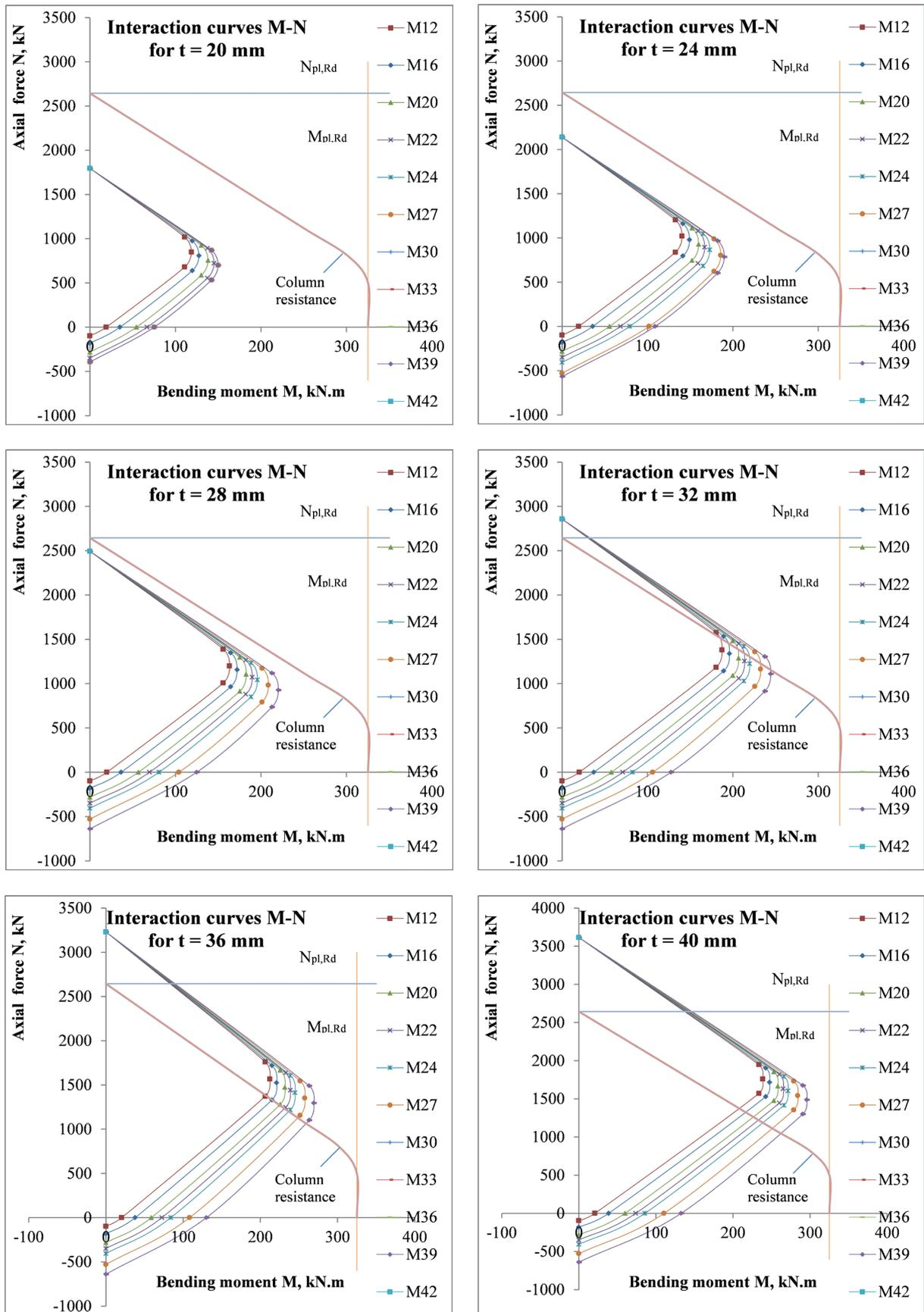
Fig. 6 M-N Interaction diagrams for different bolt diameter (Column HEA300,  $f_y = 235$  MPa; Bolt 4.8,  $n = 4$ ,  $f_{ub} = 400$  MPa; Concrete: C25/30; Base plate,  $e_a = 60$  mm,  $e_b = 80$  mm,  $e_c = 65$  mm)
