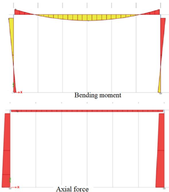
Fig. 4 Bending moment and axial force distribution of frame F1 (LC3)
