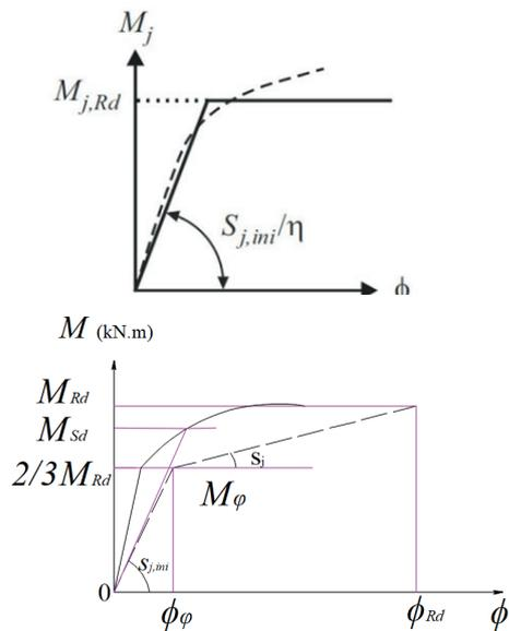
Fig. 2 Moment-rotation curves for base plate joint, a) Experimental curve [24] a) ---- Experimental curve [24]. — Idealized curve, b) ---- Modeling curve Jayarajan P. [9], — Moment-rotation curve according to EC3 [10]
