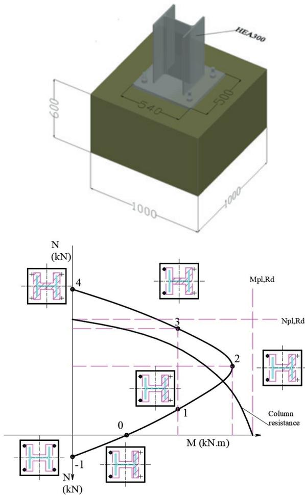
Fig. 1 Interactions diagram  $M$ - $N$  of column base bending about strong axis [15]
