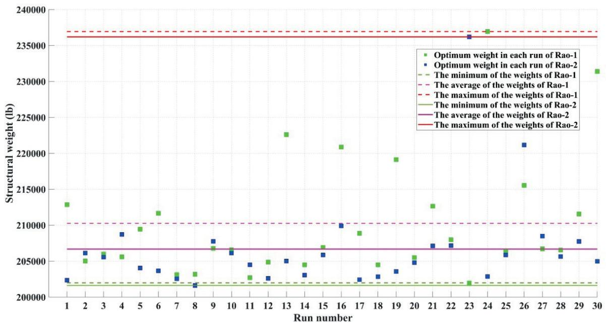
**Fig. 8** The structural weight of each independent run of Rao algorithms for the 3-bay 24-story frame structure
