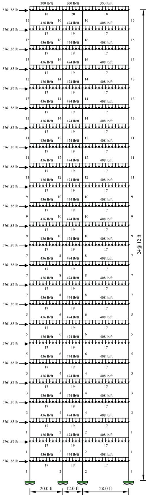
Fig. 7 The schematic of the 3-bay 24-story steel frame
