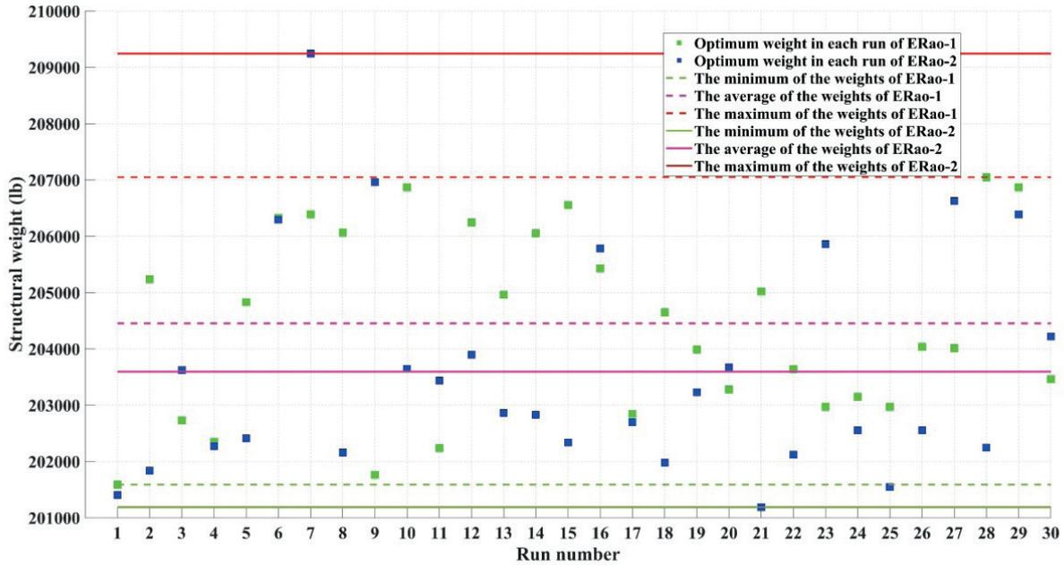
Fig. 9 The structural weight for each independent run of the ERao algorithms for the 3-bay 24-story frame structure
