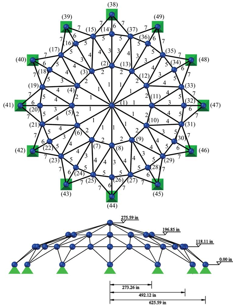
Fig. 3 Schematic of the 120-bar dome truss structure
