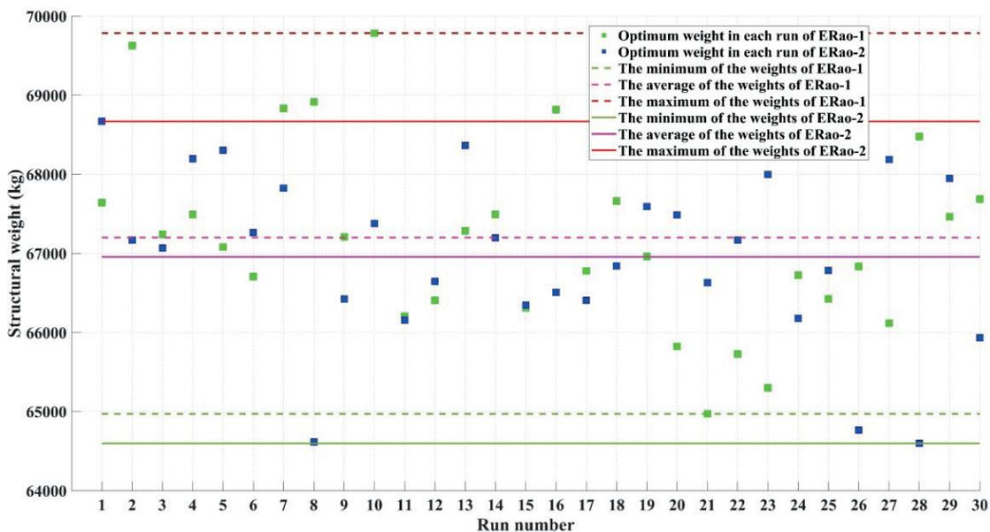
Fig. 13 The structural weight of each independent run of the ERao algorithms in the 1016-bar double layer grid structure
