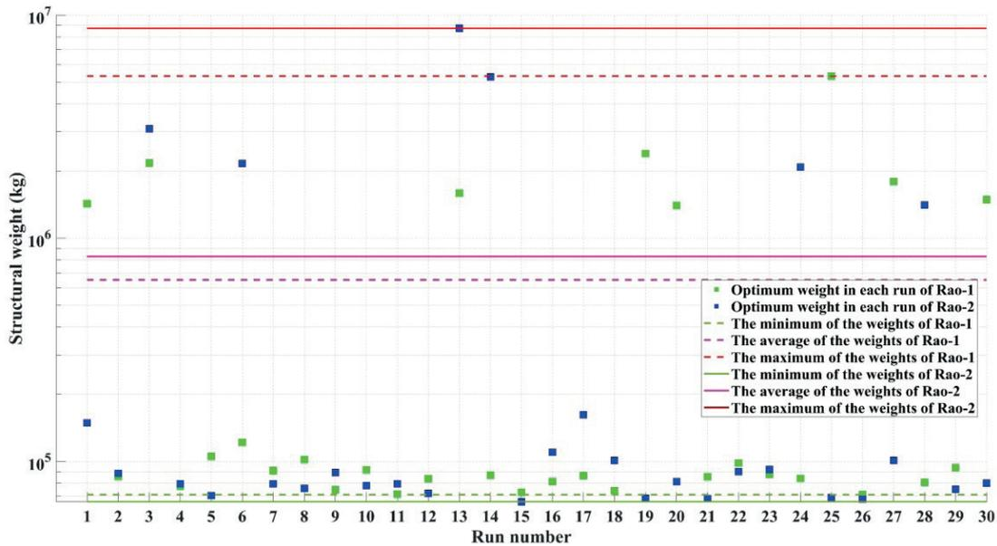
Fig. 12 The structural weight of each independent run of the Rao algorithms in the 1016-bar double layer grid structure
