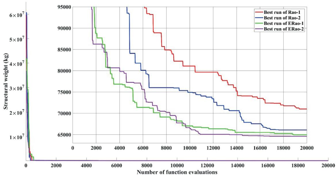
Fig. 14 Convergence histories of the best run of the Rao and ERao algorithms in the 1016-bar double layer grid structure
