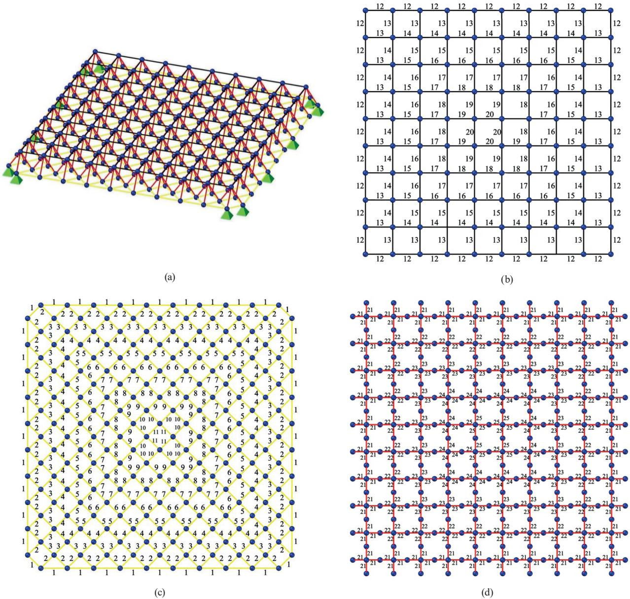
Fig. 11 Schematic of the 1016-bar double layer grid; (a) 3D view, (b) Top layer members, (c) Bottom layer members, and (d) Web members
