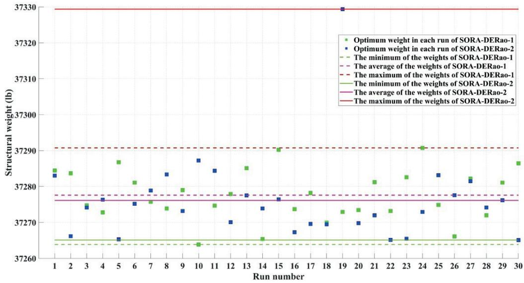
Fig. 5 The structural weight for each independent run of the ERao algorithms for the 120-bar dome truss design problem
