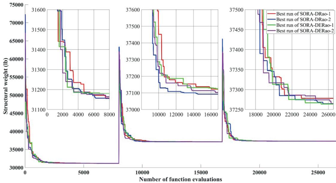
Fig. 6 Convergence histories of the best run of the Rao and ERao algorithms for the 120-bar dome truss design problem
