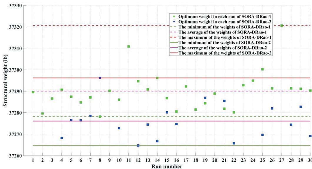
**Fig. 4** The structural weight of each independent run of the Rao algorithms for the 120-bar dome truss design problem
