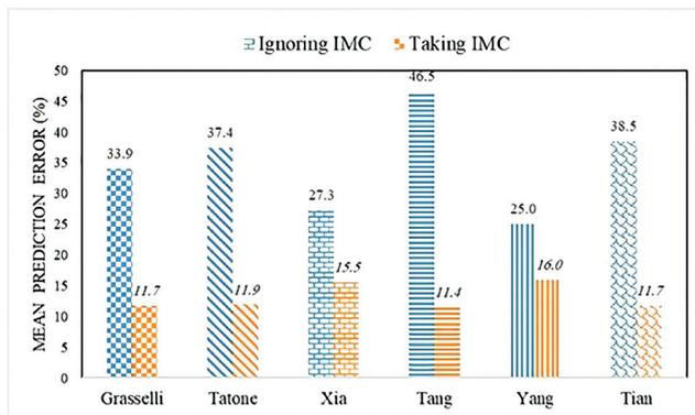
**Fig. 7** Comparative analysis of the predicted value of PSS by taking into consideration the influence of IMC on mismatched rock joints of this study
