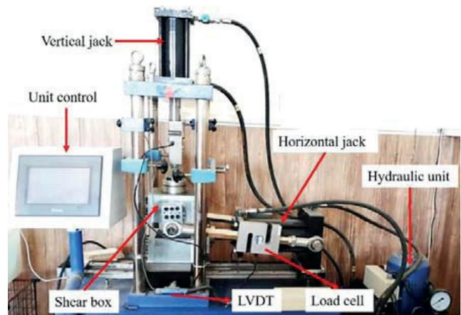
Fig. 3 Servo-controlled direct shear testing machine
