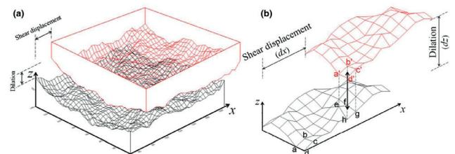
Fig. 4 a) lower and upper surfaces are defined in the same coordinate system. b) both surfaces are gridded with the same interval [21]
