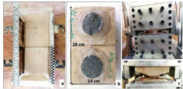
Fig. 1 Sample preparation for laboratory test: a) mold before casting, b) sample after molding and before testing, c) Prepared sample in the shear box
