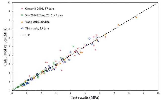
Fig. 6 Comparison between tested and estimated PSS in different models
