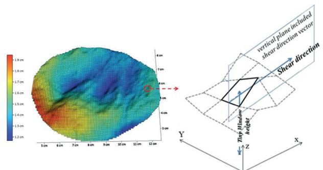
Fig. 5 Reconstructed Joint surfaces with desired/regular intervals
