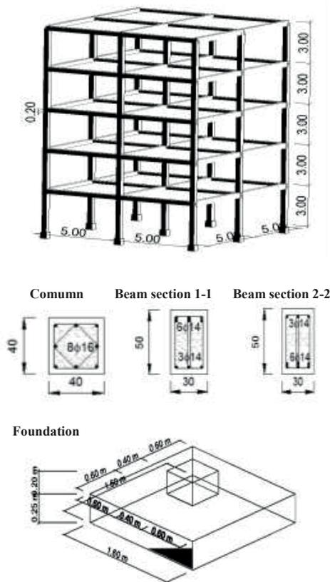
Fig. 2 Geometric characteristics of 5-story RC building
