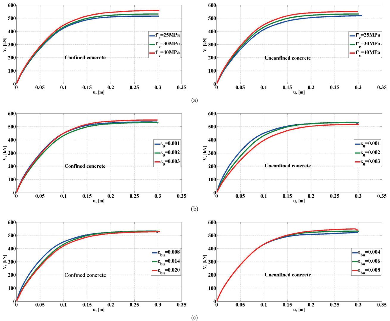
**Fig. 4** Influence of the concrete parameters of the structure on the Pushover curve; (a) concrete compressive stress, (b) peak strain corresponding to concrete compressive strength  $\epsilon_{c0}$  and (c) ultimate deformation of concrete
