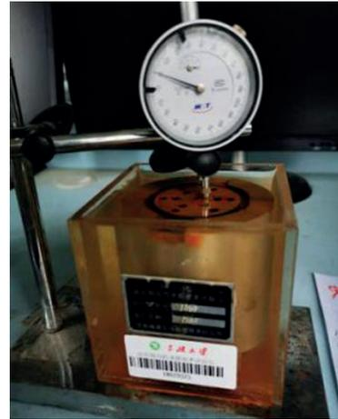
Fig. 10 The swelling test of complete mudstone Sample
