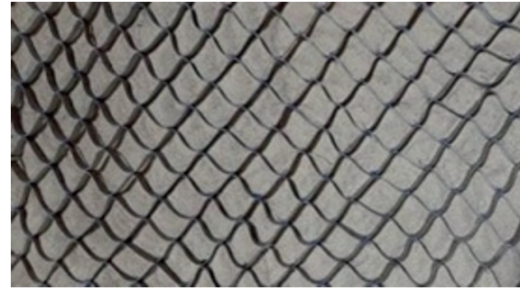
Fig. 3 Sample geocell used in laboratory model
