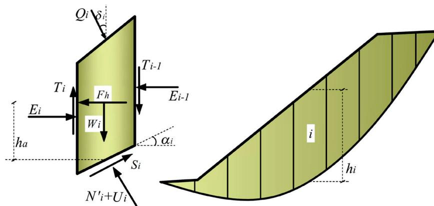
**Fig. 1** Forces acting on a typical slice,  $W$ : wight of the slice,  $S$ : shear strength,  $N$ : effective normal force,  $U$ : resultant water force,  $E$ : normal inter-slice force,  $T$ : shear inter-slice force,  $h$ : average height of the slicem  $b$ : width of the slice,  $h_c$ : height of the slice center,  $F_h$ : horizontal seismic force,  $\alpha$ :inclination of slice base,  $Q$ : external surcharge
