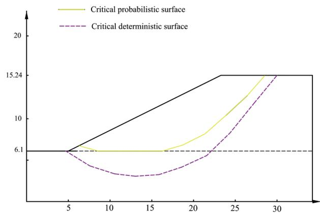
**Fig. 9** Critical failure surfaces of a multi-layered slope
