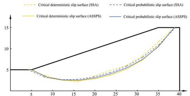
**Fig. 7** Critical slip surfaces explored by SSA and ASSPS for the first experiment
